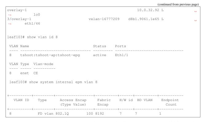
In above example, encap vlan-100 has been mapped to ACI platform independent (PI) vlan 8 which is mapped to vxlan-8192.
