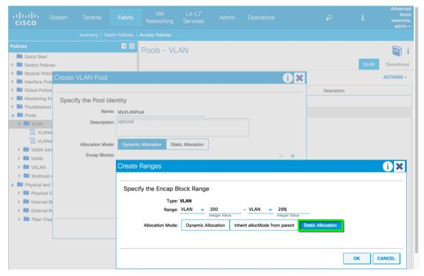
Make sure VLAN pools do not have overlapping vlans. The reason is that ACI floods STP Bridge Protocol Data Units
