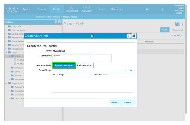
Then when you add an encap block, you can choose either static or dynamic. In that way, you will have flexibility to add both dynamic and static encap blocks. Dynamic encap blocks are used for Virtual Machine Manager (VMM) domain.
